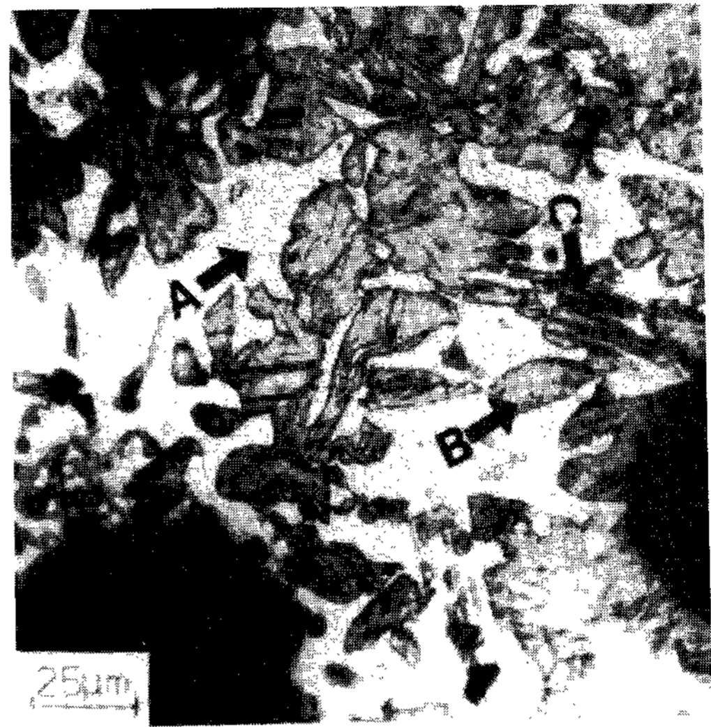
Photo 3. Microstructure showing multi-phases (ferrite-bainite-martensite) in specimen isothermally treated at 300°C for 2min after austenitizing at 860°C for 30min (5 cycles). (A) ferrite(white) (B) martensite(grey) (C) bainite(black)
