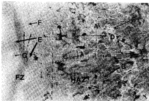
Photo. 8 Microstructure of cross section in the multilayer weldment \times 200
