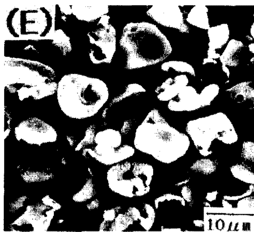
Fig. 7. Scanning electron microscopic photogram of granular structure of corn starch saccharified by mixed glucoamylase and \alpha -amylase
