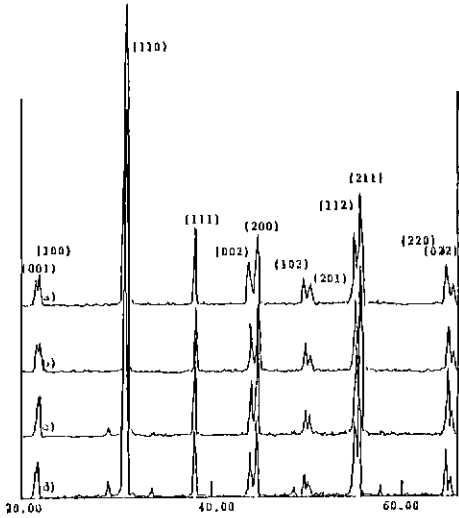
Fig. 6. X-ray diffraction analysis of various composition. (a) 4at.%Nd, (b) 6at.%Nd, (c) 9at.%Nd, (d) 12at.%Nd
