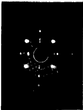
Fig.3. Laue back reflection patterns and the analysis of orientation in the ZT-2 crystal.
