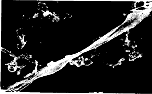
Fig. 14 SEM photomicrography of cutting wear particle( \times 350 )
