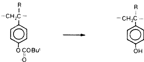
Fig. 14. Photochemistry of onium salt cationic photoinitiators and acid-catalyzed thermolysis of side-chain protecting group of poly(vinyl phenol).
