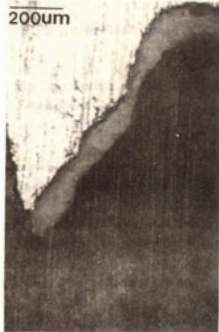
Cervical cement film thickness of shoulder with a 45° bevel preparations
