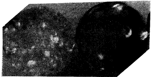
Fig. 1. Microphotograph of cation exchange resins with and without rapid freeze pretreatment(x 40), right:cation exchange resin without pretreatment, left:cation exchange resin with pretreatment.
