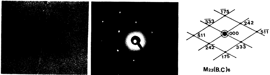
Photo. 9 TEM structure of precipitates at grain boundary of bonded interlayers
