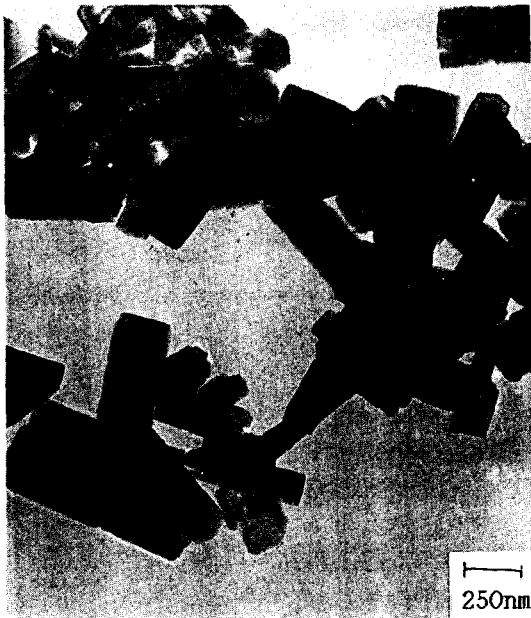
Fig. 5. TEM micrographs of synthesized ZnO powder. ( ZnCl_2 0.05mol/l , HMT 0.1mol/l )
