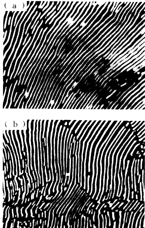
Photo 1. Microstructure of cold rolled pearlite ( \times 3,500 ).
