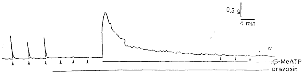
Fig 6. Effect of prazosin ( 10^{-6} M) and \alpha,\beta -methylene ATP ( 10^{-5} M) on neurogenic contraction in isolated rabbit renal artery: perivascular nerve stimulation at 50 Hz, supra-maximal voltage, 0.3 ms pulse width, for 1 sec and 5 min interval.
