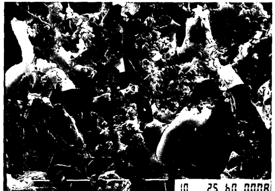
Fig.7. SEM photomicrograph showing bond failure surface of silicoated G - Cera specimen ( \times 2000 ).
