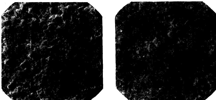
Fig. 6. Secondary electron image of carved Shofu spherical amalgam before corrosion (a) and after corrosion (b).
