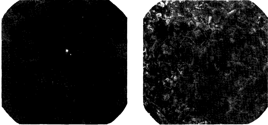
Fig. 1. Secondary electron image of polished Amalcap amalgam before corrosion (a) and after corrosion (b).
