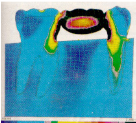
Fig. 10. Von Mises stress of Model C under P1.
