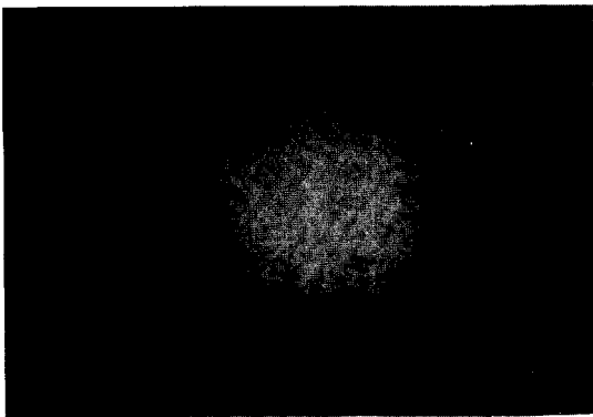
Photo. 2. Spurious interference pattern by boundary reflections.
