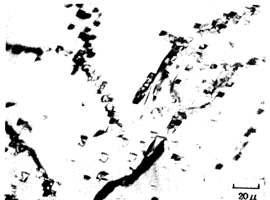
Fig. 12. Dislocation etch pits(perpendicular to growth orientation).
