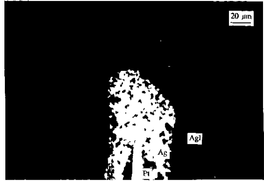
Fig. 4. Cross section of an as-prepared ionic probe.
