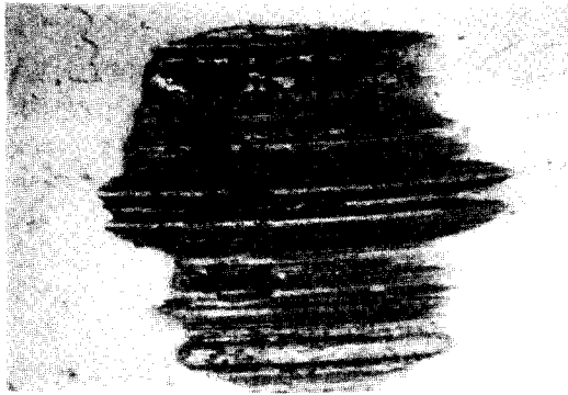
Photo 2. Micrograph of worn surface of En31 steel ball (80 μm): Neat+3.0 wt% JS
