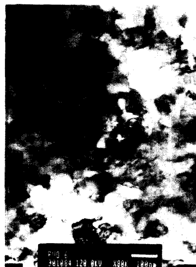
Fig. 5. TEM microstructure of 4.0 \mu\text{m} TiN coating
