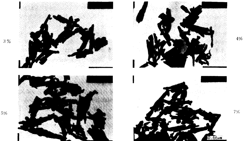
Fig. 2. TEM photographs of \gamma -Fe 2 O 3 particles coated by iron-cobalt ferrite formed depending on cobalt content (Co/ \gamma -Fe 2 O 3 wt%)
