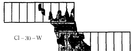
Fig 8. Corrosion shape of specimens(chloride content 0.3%, chloride water)
