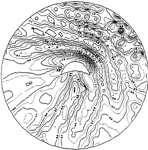
Fig. 4.6 Contour Wave Height Amplification Factor around an Emerged Semi-Circle Structure(9sec, 45° Direction, \beta=0.0 )
