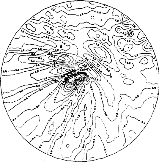
Fig. 5.16 Contour of Wave Height Amplification Factor Around a Submerged Semi-Circle Structure( \cot\theta=3.64 ) (9sec, 45° Direction, \beta=0.05 )
