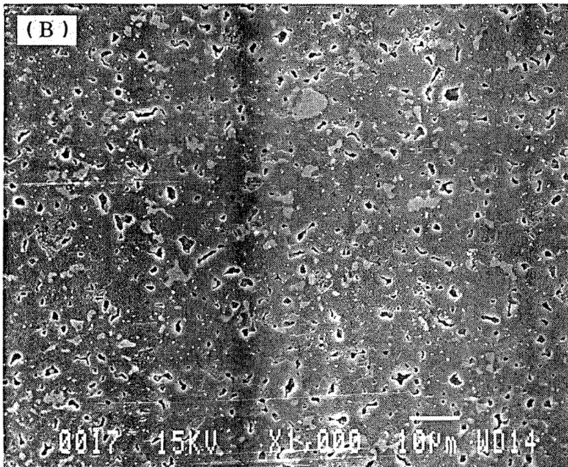
Figure 4. SEM micrographs of AlN samples sintered at 1780°C, which were prepared by (A) dry pressing and (B) slip casting.
