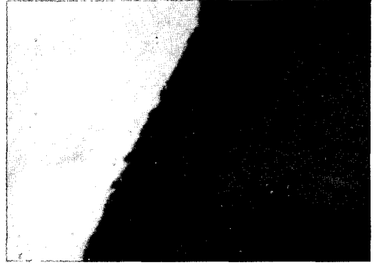
Fig. 25. Bond failure between cement and metal in fatigue test. (x 200)
