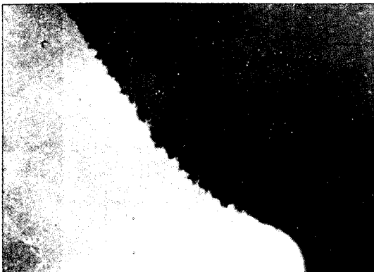
Fig. 20. Bond failure between cement and enamel in static test. (x 200)
