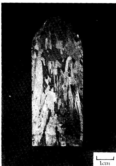
Fig. 2. Macro-etched vertical section of silicon ingot grown at a rate of 0.2mm/min.
