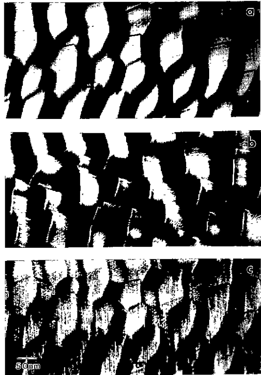
Fig. 4. A series of images from the same area shows contrast reversal of the two types of facets. (a) Only F-facets are illuminated by choosing the strong reflection spot in Fig. 3 (b) R-facets are illuminated by choosing the weak reflection spot in Fig. 3. (c) Both facets are equally illuminated by choosing both spots in Fig. 3.
