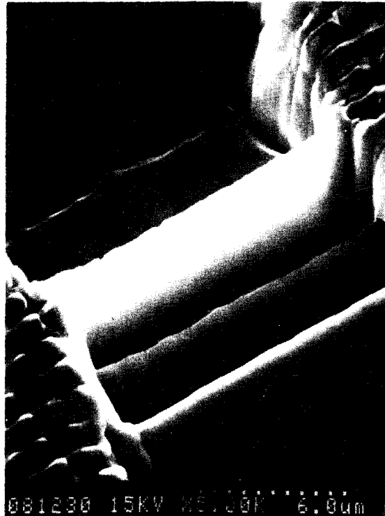
Fig. 2 Scanning electron micrograph showing the tilted view of sample prepared by focused ion beam milling.
