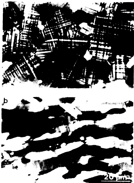
Fig. 4 Optical micrographs taken on planes (a) perpendicular and (b) parallel to the compression axis.
