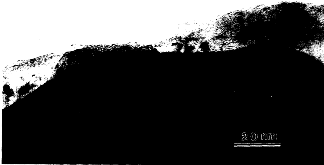
Fig. 8. Transmission electron micrographs of goethite with free carbon.
