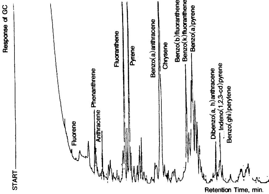
Fig. 11. Typical Chromatogram of PTFE Membrane Filter Extract.
