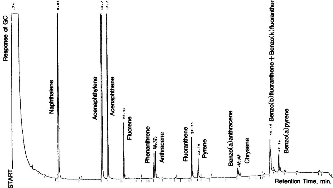
Fig. 4. Gas Chromatographic Chromatogram of PAH Standard Mixture Using Ultra 2 Capillary Column.
