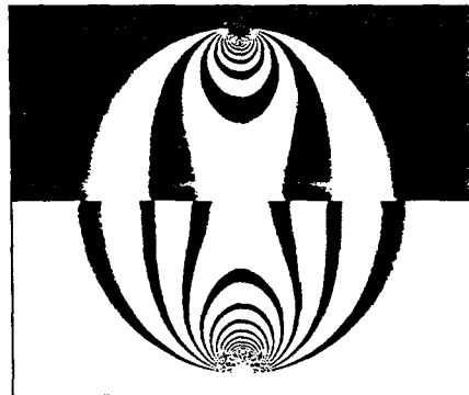
Fig. 6 Dark-field fringes(upper half) and two times fringe-multiplied pattern(lower half) generated by Eq. (4) from the computer simulated fringes of Fig. 4
