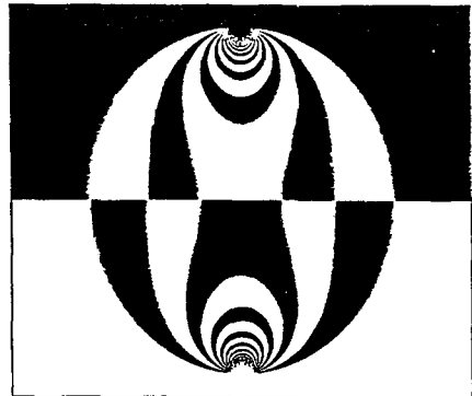
Fig. 5 Dark-field fringes (upper half) and light-field fringes (lower half) generated by Eqs. (2) and (3) from the computer simulated of Fig. 4
