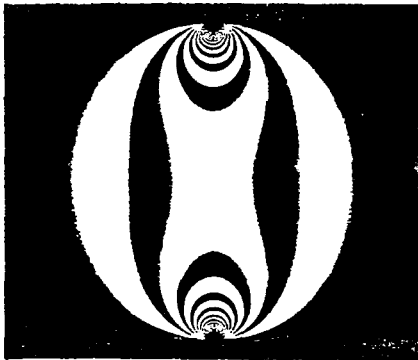
Fig. 4 Computer simulated photoelastic isochromatic fringe pattern of a disk compressed by two diametrically opposite concentrated loads in a dark-field circular polariscope arrangement (simulation data : P=8.90 N, R=2.286 cm, t=0.476 cm, f_\sigma=3.503 N/cm)
