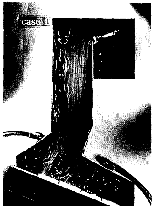
Fig. 7 Streamlines for a counter flow type incinerator (case C3)
