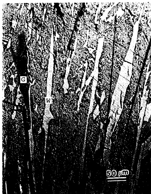
Fig. 5. Microstructure of the annealed \text{YBa}_2\text{Cu}_7\text{O}_x sample ( 200\times ); (G) \text{YBa}_2\text{Cu}_3\text{O}_x and \text{Y}_2\text{BaCuO}_5 , (W) \text{CuO} .
