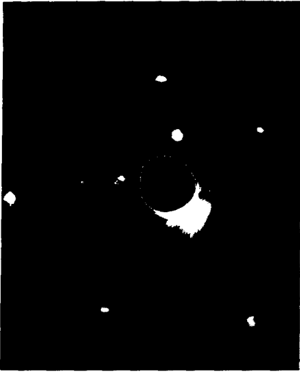
Fig. 8. Laue back reflection pattern of [0001] direction grown rod shaped single crystal.
