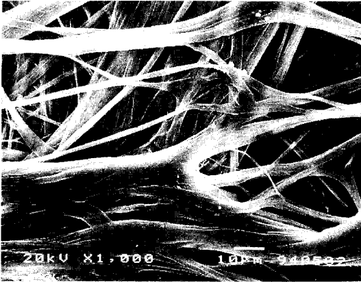
Fig. 3. Scanning electron micrographic photo of polyethylene fibers chemically treated after using fibrous beds.
