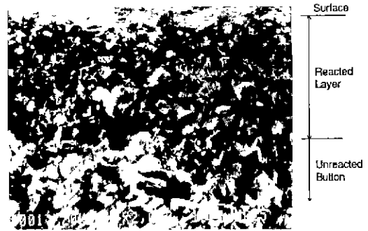
Fig. 3. SEM photo of interface between reacted and unreacted region of skid button.
