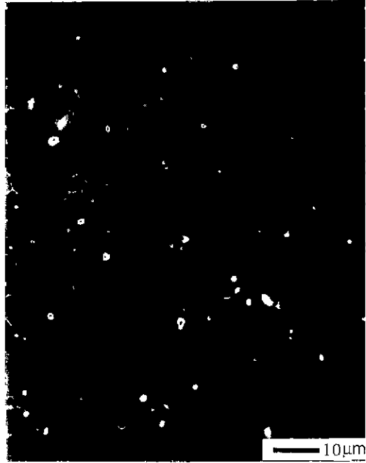
Fig. 2. SEM micrograph of the alumina specimen after thermal etching at 1500°C during 1 hr.
