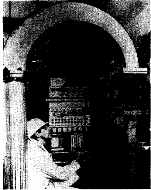
Fig. 1 Test section, tube bundle, instrumentation and outlet piping of two-phase vibration test loop
