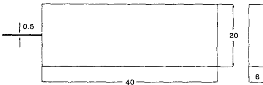
Fig. 2. Dimension of test specimen(unit : mm).
