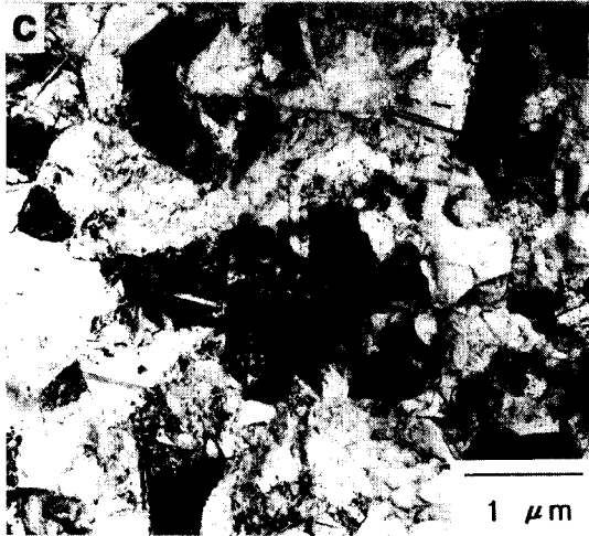
Fig. 8. A series of plan-view TEM micrographs of the \text{Si}_{0.47}\text{Ge}_{0.53} film annealed at 550^\circ\text{C} with the annealing times of (a) 10min, (b) 30min, and (c) 1hr.
