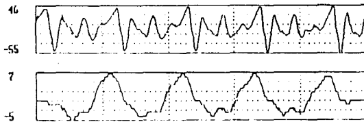
Fig. 3-1 G-peak detection using second-order variable bandwidth LPF. (a) Speech signals (b) The waveform through second-order variable bandwidth LPF
