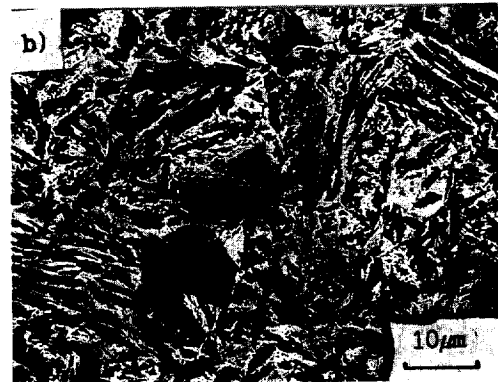
Photo. 1 Untempered microstructure of SCM 440 steels austenitized at 855°C, a) oil cooling, b) Compressed air cooling
