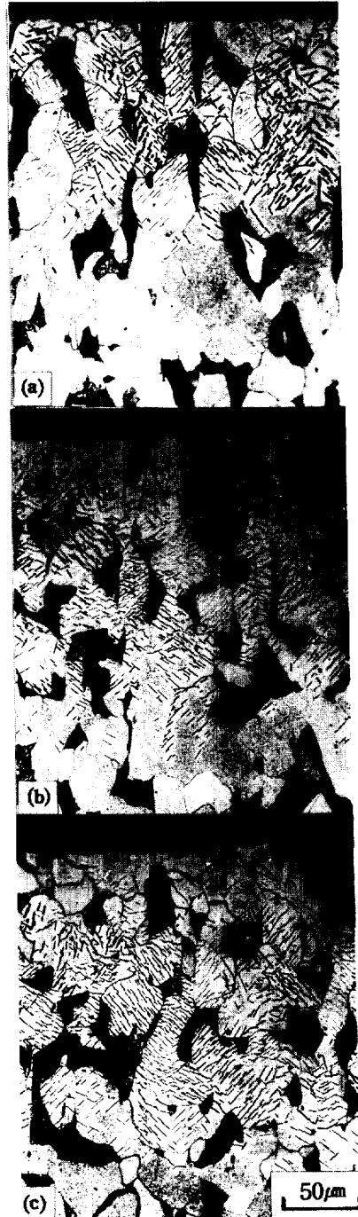
Fig. 5 Optical micrographs showing the depth of diffusion zone of SM20C steel aged at 450°C for 1hr after oxynitriding at 570°C for 2hrs in 50%NH 3 + Air + N 2 atmospheres with various addition of air : (a) 9% (b) 27% (c) 36%
