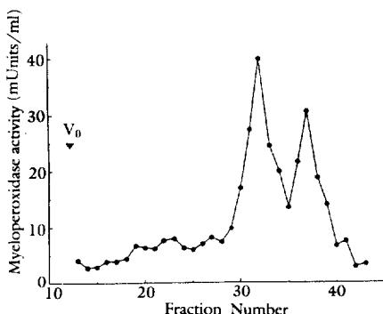
Fig 4. Sephadex G-200 gel filtration of myeloperoxidase.  $V_0$ : void volume
