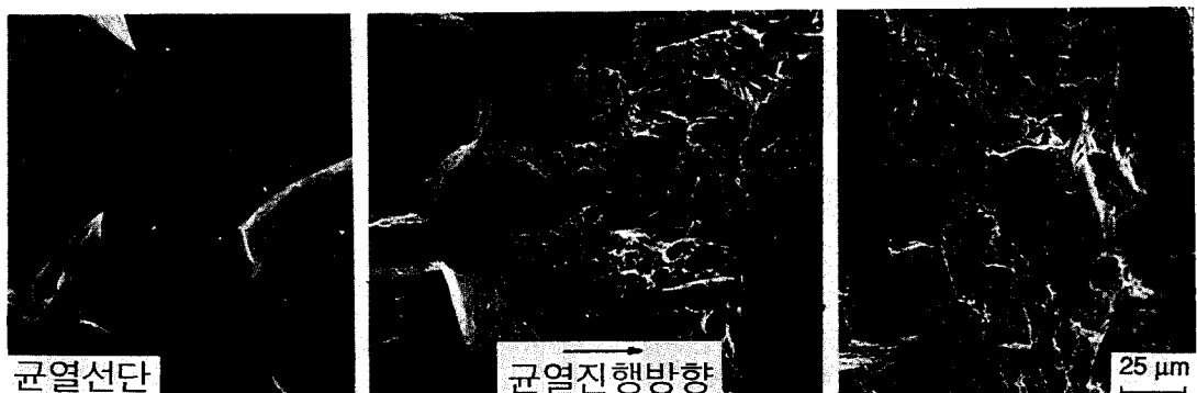
Fig 11. Transition of reheat crack of the heat affected zone flrom 1150°C single cycled
