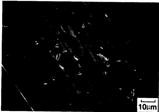
Photo 3 Microstructure of stainless steel containing 25 ppm B after Strauss test.
