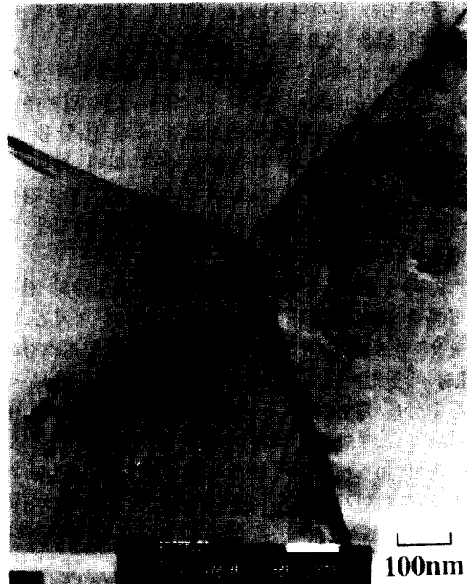
Photo 4 TEM micrograph of grain boundaries for stainless steel containing 25 ppm boron in as-received condition.
