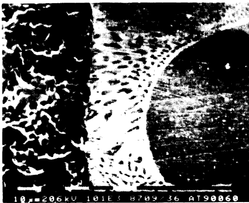
Photo. 2. Microstructure of the interface brazed by AT alloy at 950°C for 1.8ks.
