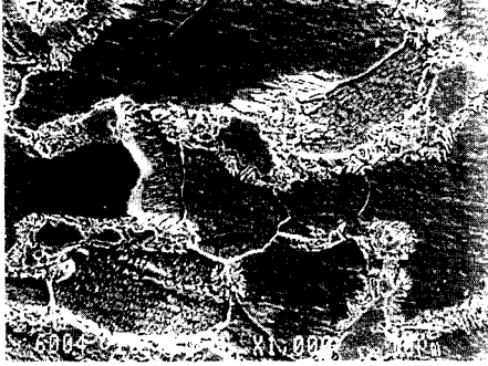
Fig. 5 Macrostructure of heat-treated low carbon steel
